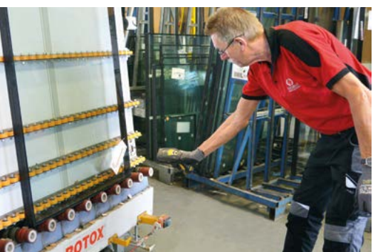
Thanks to bar code registration, the location of each insulated glass unit in the glass buffer is known. Workers on the glazing line scan the label on the frame or sash. The sheet is then guided by the A+W Cantor system out of the buffer and to glazing: a secure system without the need for searching.
