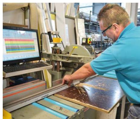
Networked throughout: Even the manual workstations are equipped with CIM production monitors.
