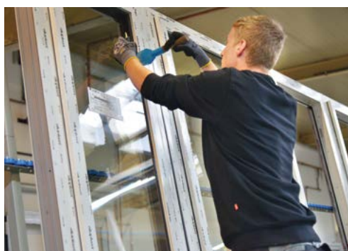
Thanks to bar code registration, the location of each insulated glass unit in the glass buffer is known. Workers on the glazing line scan the label on the frame or sash. The sheet is then guided by the A+W Cantor system out of the buffer and to glazing: a secure system without the need for searching.
