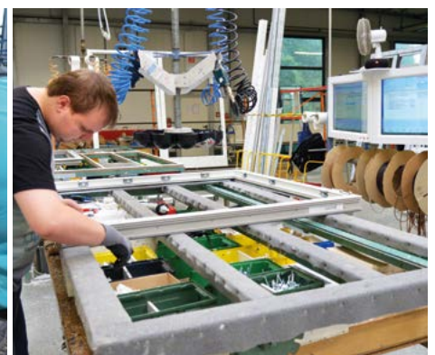
Networked throughout: Even the manual workstations are equipped with CIM production monitors.
