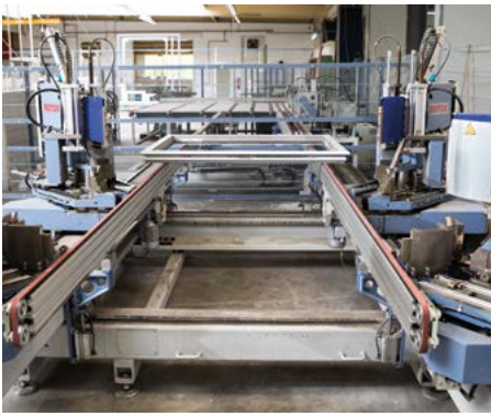
Automatic transport lines convey the frames and sashes between the processing stations, here from welding to polishing.
