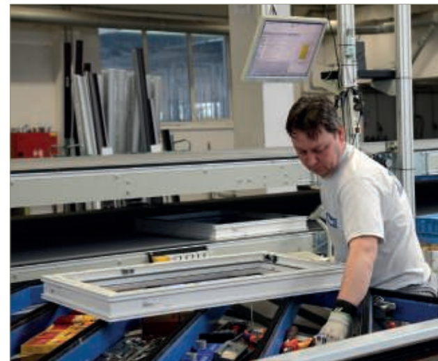
Left: Michal Buzna, responsible for acquisitions and project management at INCON during inspection of a complex component. Right: With bar code reading, the worker at this fitting station has displayed the production information for the current workpiece on the monitor, thus sparing him the need to use the traditional production paperwork. Clearly visible in the background: The automatic conveyor that transports the machined element to the buffer.
