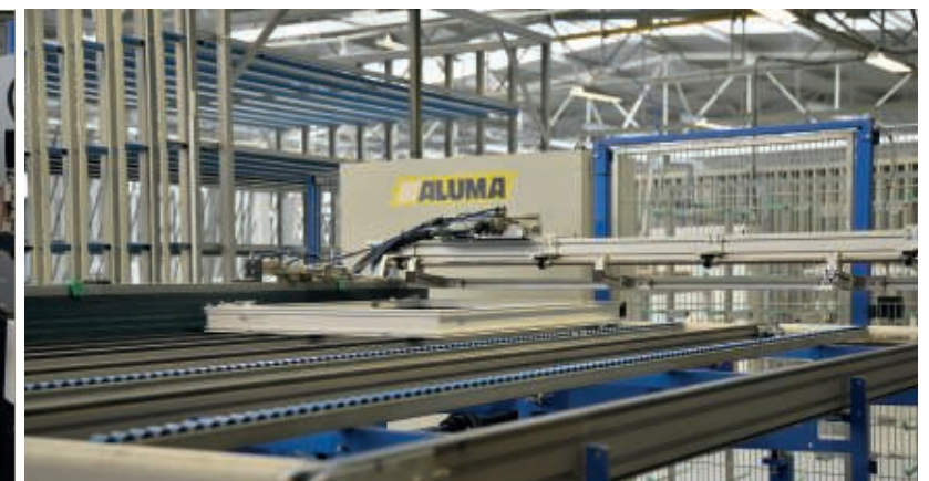
At the end of the automatic transport path, the components are raised and placed in a vertical buffer.
