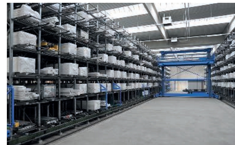
Intelligent material management in window construction: Fully-automatically controlled profile stores
