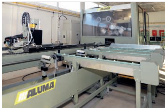
Left: Bar processing in aluminum production: The CANTOR-controlled Quadra L1 completes all drilling, milling, and cutting tasks with speed and precision. Right: Solid skilled work and years of experience enable production of aluminum components with perfect functionality and flawless finish like this lift and slide door.
