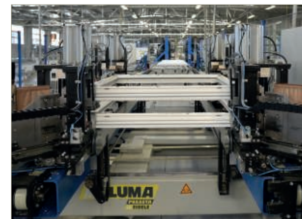
Fully automatic welding on the horizontal Double-Stürtz welding machine. For frames and casements, INCON runs two parallel production lines; intelligent buffers help to make sure that the „couples“ are united at the „wedding“ even if one of them should arrive later than planned.
