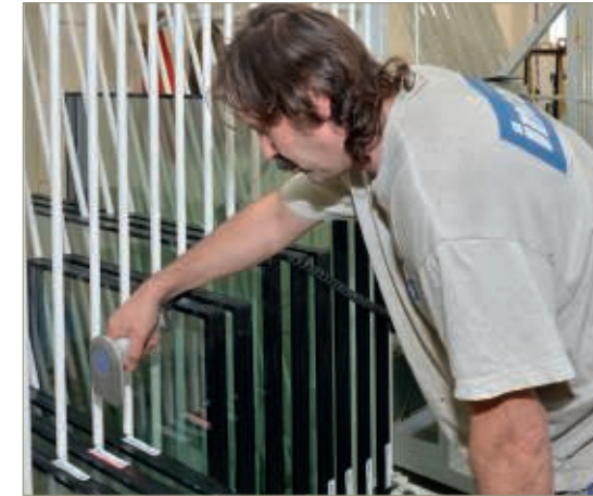
Left: In goods receiving, each individual insulating glass unit is posted to a defined rack. Now it is known in the system where it is and which component it belongs to. Right: After reading the bar code of the label on the casement, the worker in glazing sees the rack of the associated insulating glass unit displayed on his workstation monitor – thus virtually eliminating errors.
