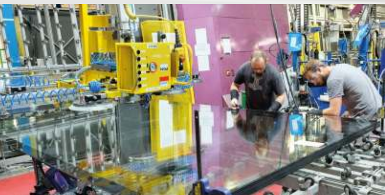
Not everybody can produce sheets like this: three-layer, large format stepped IGU
