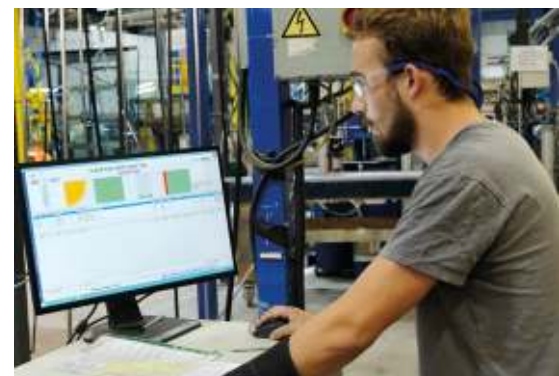
A+W Production Monitor on the inspection point of the insulated glass line: sheet structure, position and correct orientation of the layer are clearly displayed
