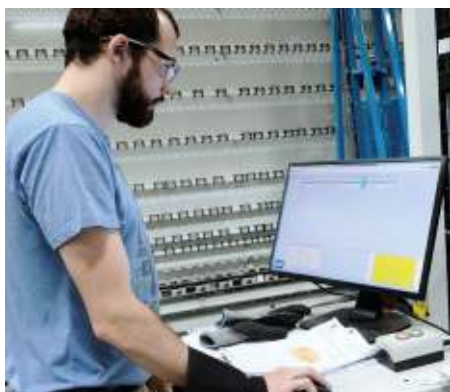
Controlled via network: an A+W Production monitor on the vertical LSG cutting line
