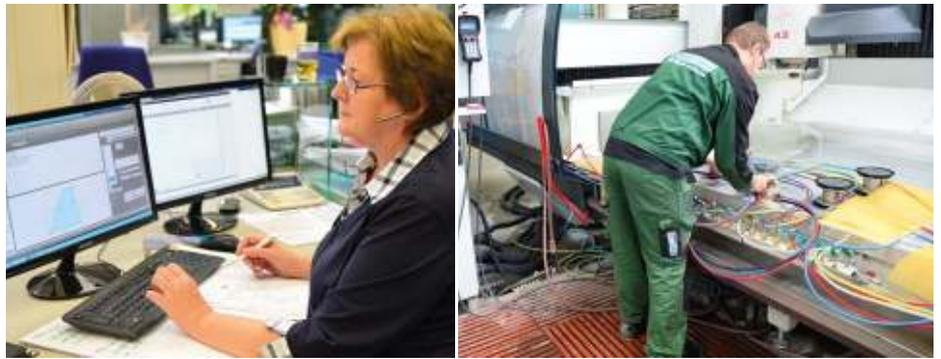
The DXF files are transmitted online to the CNC centers and the Schraml drilling machine. The machine operator scans the sheet label and then sees all technical data for the sheet such as dimensions, processings to be done, etc. on the A+W Production Terminal. If everything looks right, he initiates processing.
