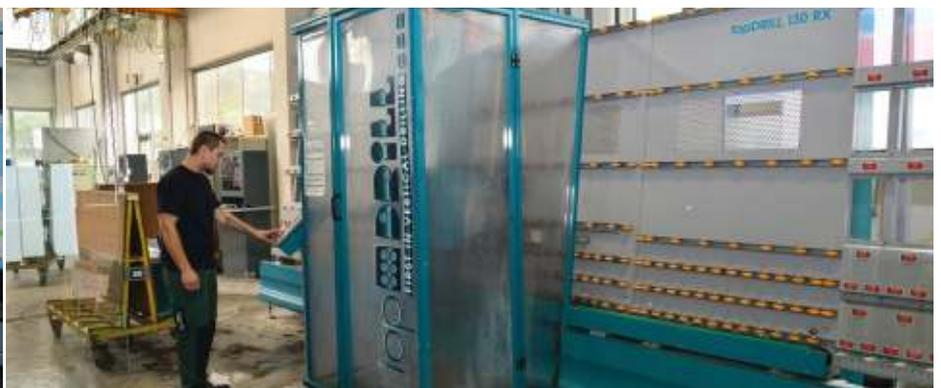
With a bar code reading, the machine operator on the Schraml drilling machine displays the data (dimensions, processings) for the current sheet on the A+W Production Monitor. There is no programming to do since the A+W high-tech interface makes the finished control data available: thus it is also possible to produce a lot size of 1 economically.
