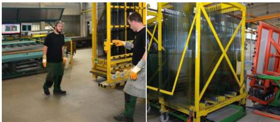
The greatest efficiency in cutting, sorting, and insulated glass feeding: the automatic insulated glass feeder (right) is the ideal complement to automated sorting with the HEGLA SortJet, which is controlled by A+W Dynopt.
