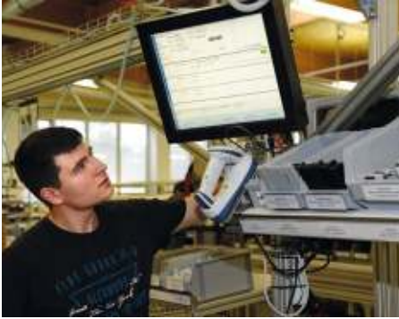
Paperless and reliable: A+W Cantor production monitors inform workers at each workstation about products, status, and intended processing.
