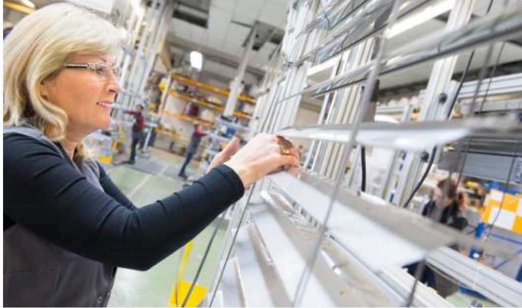
Venetian blind production at Schlotterer. Thanks to the RETROLux slats, the heat stays outside, while valuable sunlight is directed into the interior of the room.
