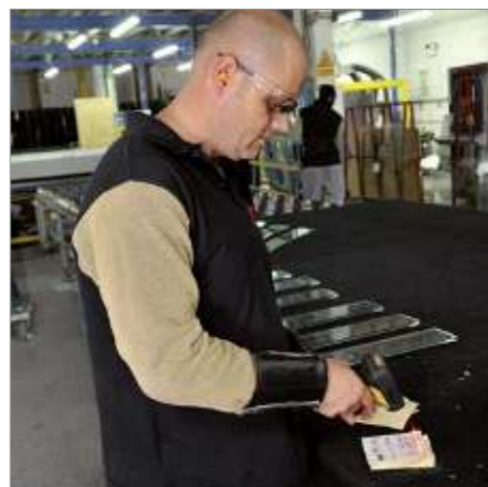
Using A+W barcoding, the status of each pane is registered in the production system and in the order processing – customer inquiries and evaluations by the management are supported optimally.
