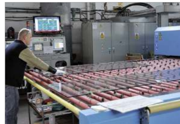
Left: The A+W Production Monitor shows the bed configuration at the infeed of the high-tech toughening furnace so that space is saved – the oven capacity is used optimally, up to 900 square metres of glass per shift are hardened. Naturally soft coatings, ornament and low-iron glass of the highest quality can also be toughened. Right: The modern Bottero CNC centre allows all edge processing and holes, even on model panes and free shapes.
