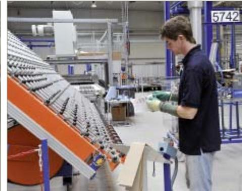
With just a few exceptions, this is the only production paper at Semcoglas Glastechnik: the label. It contains all information for identifying the sheet and track its way on the shop floor. Barcode registration at the exit of the grinding/drilling/milling line is used to report processing of the sheets complete, and assign them to the next technology.
