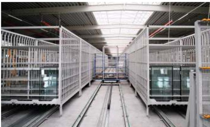
The completely automatic glass buffers feed the insulated glass units in along with the elements for glazing
