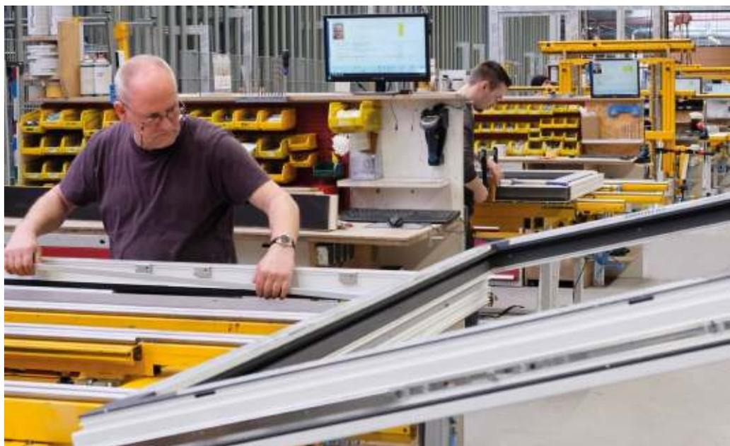
Special construction workstations where elements are automatically fed to the manual workstations
