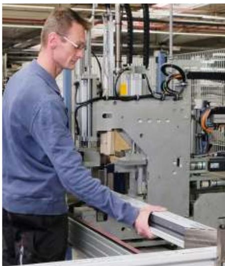
Four Rotox four-head welding machines operate the production lines at minute intervals
