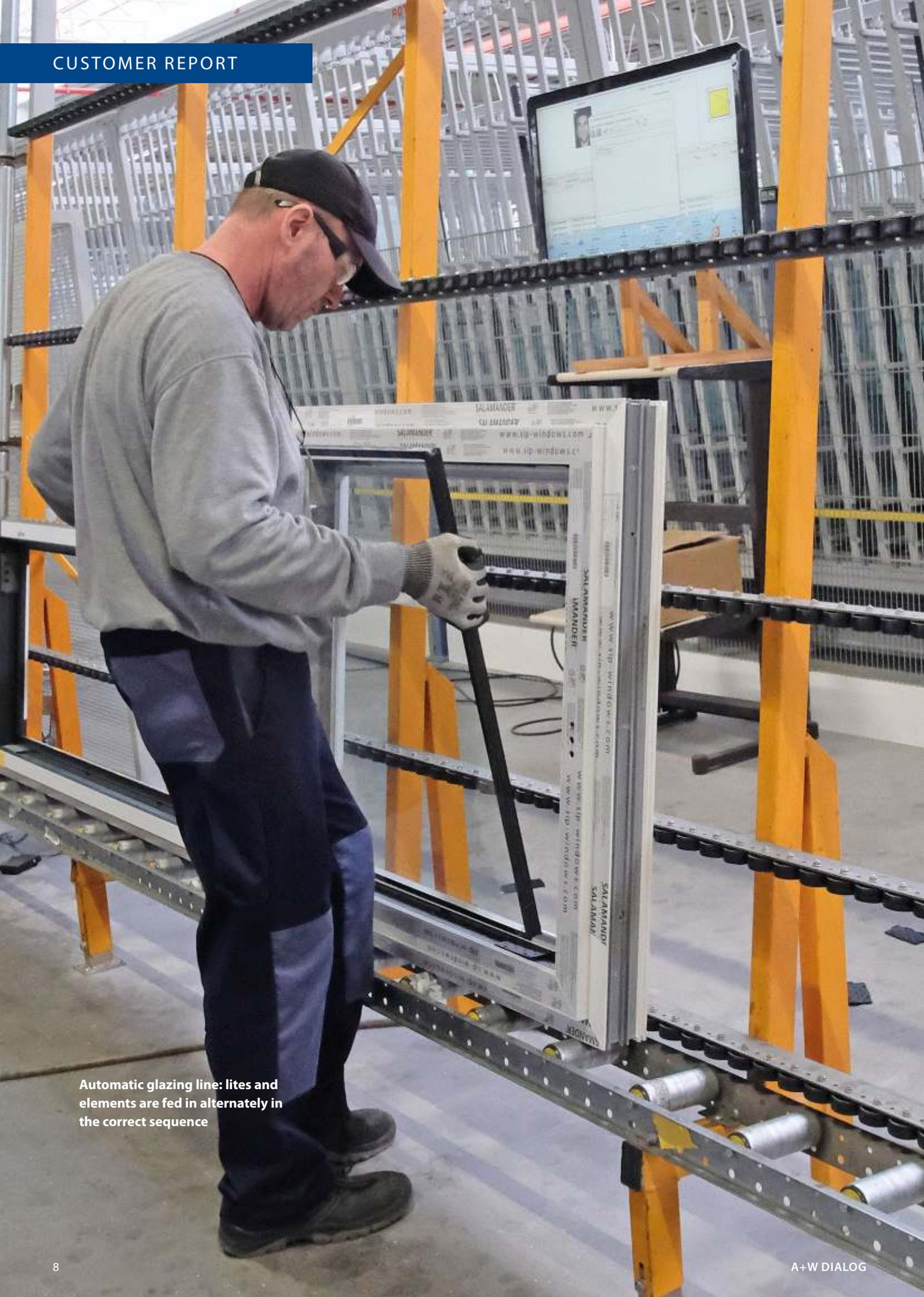
Automatic glazing line: lites and elements are fed in alternately in the correct sequence
