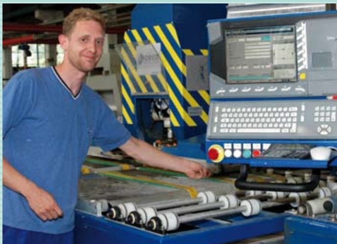
CNC drilling in networked production environment: The ToolTV control unit shows the man at the machine the sheet geometry and production data – sheets are identified by scanning their barcodes. After a brief check, the operator scans the barcode again and thus releases the transfer of CNC data: fully automatic processing begins.
