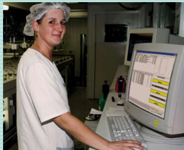
In the laminating clean room, ToolTV shows the parameters of the current pair of sheets, the sheet structure, and especially the film layer to be used. Before the sheet is passed on to the pre-compound, the operator reports it complete by scanning its barcode.
