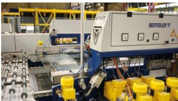
Outstanding throughput and exact edge processing for CURA Glass LSG: the new Benteler CNC processing center
