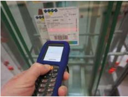
The label includes all necessary lite information. The lite status can be booked paperlessly in the ERP system A+W Business thanks to a simple barcode reading
