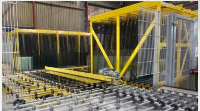
The sorter, intelligently controlled by A+W software, ensures reliable just-in-time production and constant feeding of the Benteler processing center
