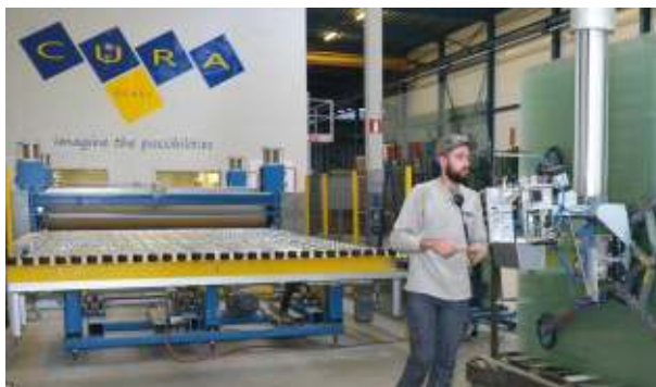
Intake of the fully automatic Benteler lamination system. Approx. thirty film types are constantly available for use.
