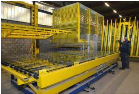
Top: fully automatic Hegla-VSG cutting system with compact warehouse and VSG-Remaster. Right: The A+W Realtime Optimizer is used to optimize and trigger the Jumbo plates from the compact warehouse and the cuts in the Remaster according to the situation.
