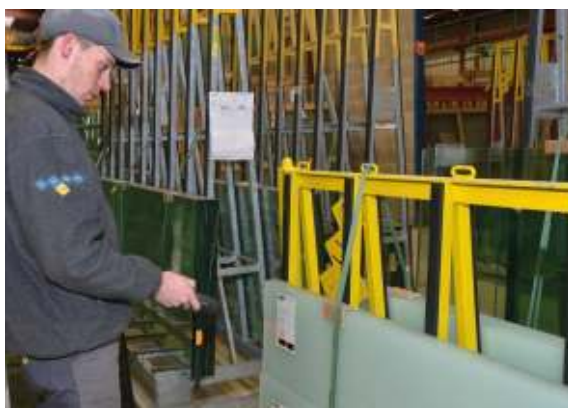
Modern internal logistics: thanks to continuous barcode registration, the position and the processing status of every pane are filed in the A+W Production database and can be called up per mouseclick.
