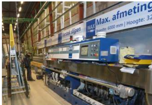
High-speed edge processing with the Bovone sanding line, from small panes through to float glass.
