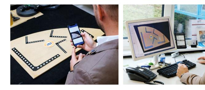
For production of a non-rectangular sheet (shape, free form), glass processors frequently receive a hand drawing or a wood, chipboard or cardboard template from the customer. Modern production on CNC machines requires digital data in order to define these shapes.
