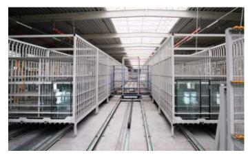
The completely automatic glass buffers feed the insulated glass units in along with the elements for glazing
