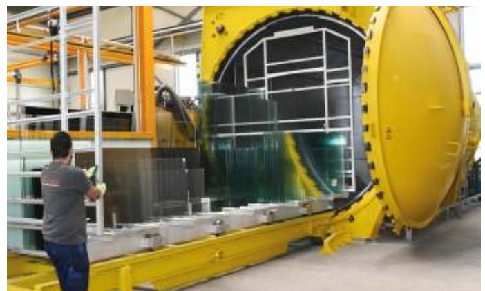
Completely "baked": laminated glass lites are transported out of the autoclave
