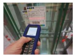
The label includes all necessary lite information. The lite status can be booked paperlessly in the ERP system A+W Business thanks to a simple barcode reading
