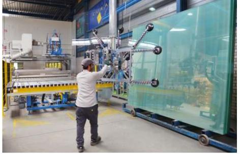
Laminated glass from jumbos: intake of the fully automatic Benteler LSG production line
