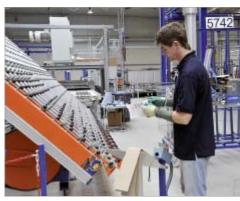
With just a few exceptions, this is the only production paper at Semcoglas Glastechnik: the label. It contains all information for identifying the sheet and track its way on the shop floor. Barcode registration at the exit of the grinding/drilling/milling line is used to report processing of the sheets complete, and assign them to the next technology.
