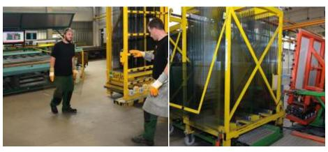
The greatest efficiency in cutting, sorting, and insulated glass feeding: the automatic insulated glass feeder (right) is the ideal complement to automated sorting with the HEGLA SortJet, which is controlled by A+W Dynopt.
