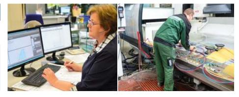
No detours in production: technical order entry with A+W Business. The data for the CNC machines is generated during order entry and provided to the machine on the A+W Production Terminal.
