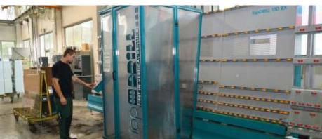
With a bar code reading, the machine operator on the Schraml drilling machine displays the data (dimensions, processings) for the current sheet on the A+W Production Monitor. There is no programming to do since the A+W high-tech interface makes the finished control data available: thus it is also possible to produce a lot size of 1 economically.
