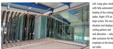
with fully automated loading of the cutting tables. Right: XTV on large screen. The visualisation tool displays cutting pattern and rack allocation - valuable assistance for the employee at the break-
