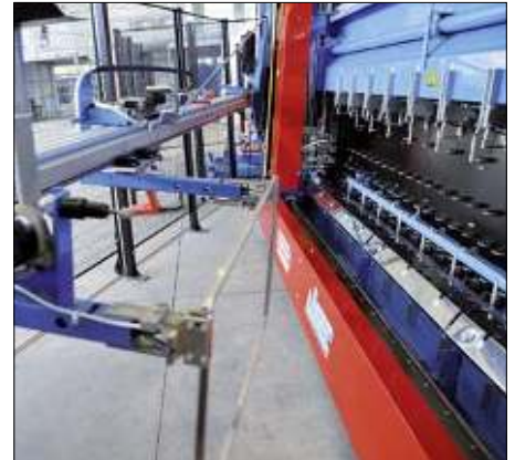
Automatic spacer application at the LISEC high-performance IG line. All modules of the line communicate with the cutting line via ALBAT+WIRSAM software to guarantee quick reactions to any change of production sequence.
