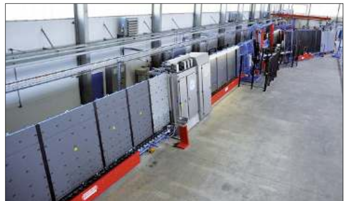
Right: The LISEC line does its job, software-controlled, and mainly without any human support – the shop floor practically empty, a strange view. Left: at the checkpoint, the ALBAT+WIRSAM monitoring system ToolTV shows sheet structure, sizes, and position of layers. Labels are printed right at the line. The printing sequence is automatically adapted to any changes in the production sequence..
