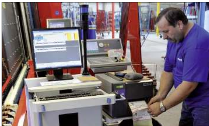
Right: The LISEC line does its job, software-controlled, and mainly without any human support – the shop floor practically empty, a strange view. Left: at the checkpoint, the ALBAT+WIRSAM monitoring system ToolTV shows sheet structure, sizes, and position of layers. Labels are printed right at the line. The printing sequence is automatically adapted to any changes in the production sequence..
