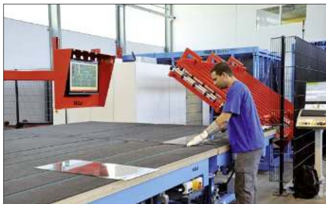
Far right: The buffer of the HEGLA Sort-jet with unloading shuttle, the link with the IG line at the bottom right. In the background: the turning device, Re-master, and portal crane. The unloading shuttle can take three sheets at once which makes the creation of sequences for producing triple IG much easier. Inside right: At the breakout table, the sheet is aligned with a stopper then set up vertically for being loaded into the sorting buffer.
