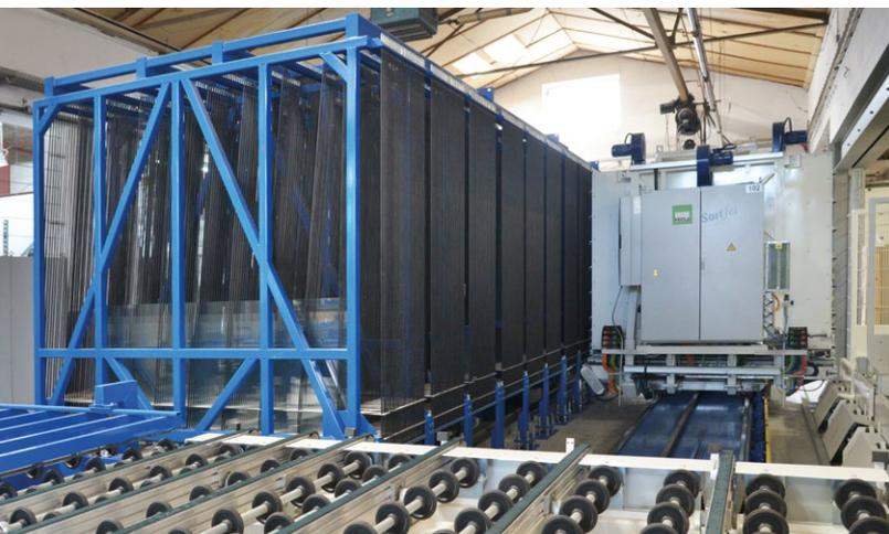
Cutting with the highest performance, minimal waste, and desired sequence for IG and processing: the sorting system controlled by A+W DynOpt was custom-tailored for Teutemacher’s complex requirements.
