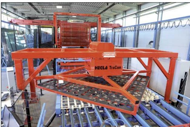
Left: Straight ahead! Fandel are the first to use HEGLA's subplate turning device TraCon. With this space-saving development there is no need for a 90° change of direction on the transport belt between X- and Y breakout.
